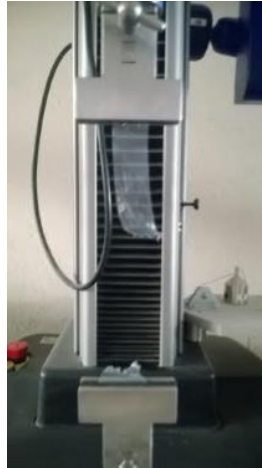
Illustration 1. Sample M1 in the universal machine before the study began.
