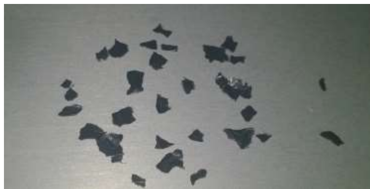
Illustration 4. Sample C-3 at 2% after 441 days of study
